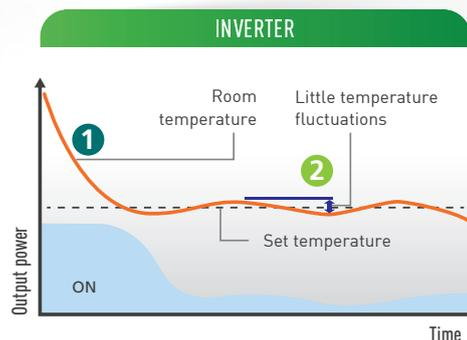
NOTE: Saves energy by varying the rotation speed of the compressor to maintain the set temperature.
